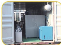
■ 后视图：气源、调直机 Back view: air supply, wire straightening machine
